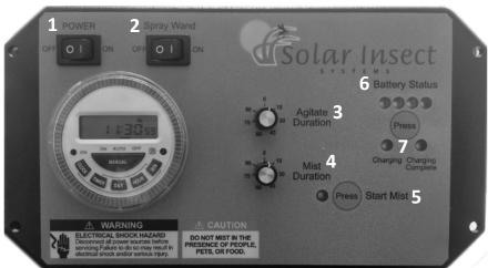
3. AGITATION DURATION - purges trapped air from the Pump head and agitates the solution in the Cube prior to a mist cycle. The recommended amount of agitation duration for a 55 gallon tank is 30 seconds. **NOTE: The minimum amount of time to purge trapped air from the Pump head is 5 seconds.**
