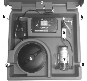
2. WIRE RECESS - Insert the two pin connector from the Battery Charger in through the center top opening **from the back of the Cube**, and attach it to the mating two pin connector (3) coming off the Battery. Plug the Battery Charger into a 120v outlet.
