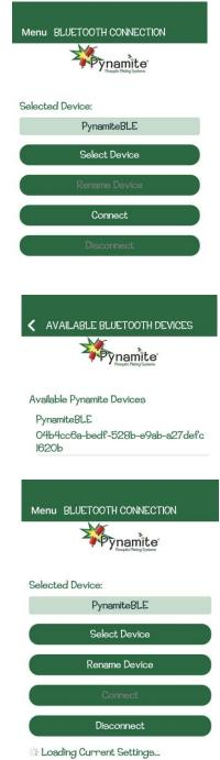
**Disconnecting the Device**: Press the Disconnect button to disconnect the app from the selected device. This button is disabled if no device is connected.
