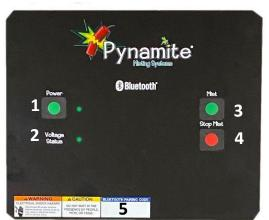
1 POWER - Press the Power button to turn the system ON or OFF. The green LED indicates the system is ON. <u>NOTE:</u> The power to the Power Supply must be plugged in and turned on as well. <u>NOTE:</u> The app default is 0 nozzles, the system will not mist until the controller is paired and the nozzle count is increased to at least 1 nozzle in the set-up screen.
