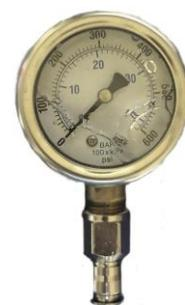
The pressure tester can also be used along the nozzle circuit to check for leaks. To attach the pressure tester to the nozzle circuit, remove a nozzle and adapter from the fitting and insert the tubing attached to the pressure tester into the fitting that was holding the nozzle and adapter.
