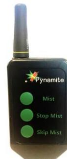
Learn Optional Transmitter: is used to pair a handheld remote.
