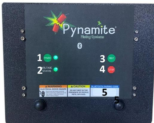
1. POWER - Press the Power button to turn the system ON or OFF. The green LED indicates the system is ON.
